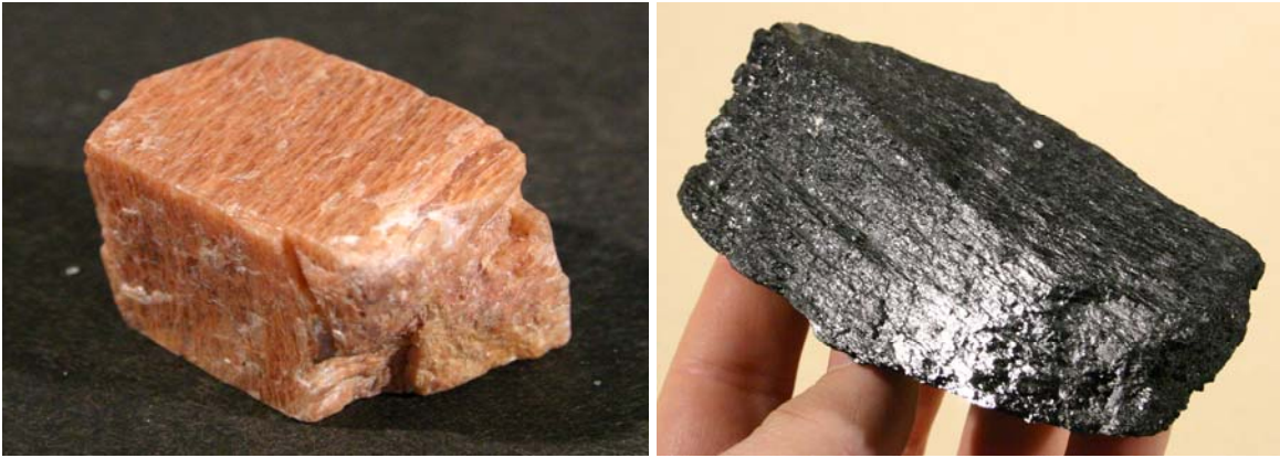
Figure 10: Two directions of cleavage: A. Cleavages in potassium feldspar intersect at 90^\circ ; B. Prismatic cleavages in hornblende intersect at 56^\circ and 124^\circ .
