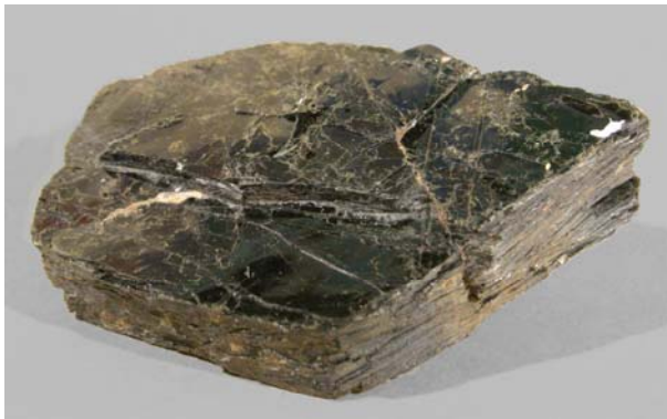
Figure 9: The mineral biotite has basal cleavage, meaning it has one perfect cleavage. The cleavage plane is apparent in the flat, reflective surface on top of this sample. The flat surface on the bottom, in contact with the table top, is parallel to the top and therefore represents the same plane of cleavage.
