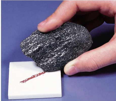
Figure 3: The streak of this dark gray mineral (hematite), obtained by rubbing it on the white streak plate is reddish brown.
