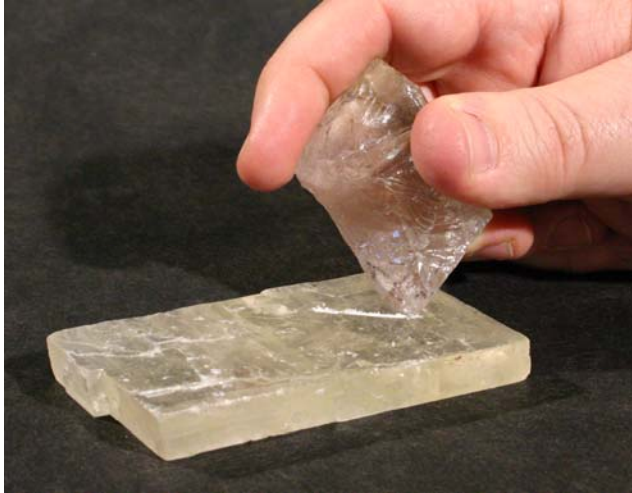
Figure 4: Testing mineral hardness. The harder mineral (quartz) scratches the softer one (calcite).
