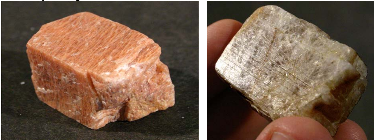
Figure 19: The thin veinlets seen in some potassium feldspars (left) should not be confused with striations in plagioclase (right). Striations are visible on the upper surface of this sample of plagioclase.
