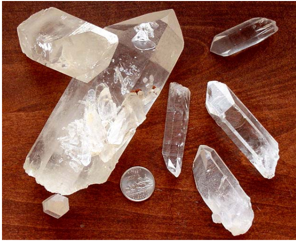
Figure 15: Crystal of quartz. Sides form a hexagonal prism that is capped with pyramid-like faces. Note the fine grooves on some crystal faces.
